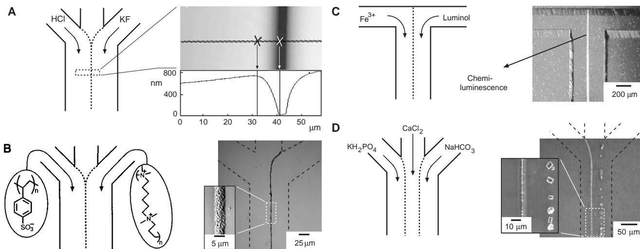
**Fig. 2.** (A) Atomic force microscopy profile of a trench (half-width = 6 μm) in SiO<sub>2</sub> on a Si wafer etched by HF that is generated on the interface of laminar flow of KF (2 M in H<sub>2</sub>O) and HCl (2 M in H<sub>2</sub>O). (B) Optical micrograph of a polymeric structure deposited on glass at the laminar flow interface of 0.005% aqueous solutions of poly(sodium 4-styrenesulfonate) and hexadimethrine bromide. (C) Optical micrograph of
