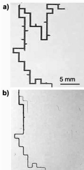
**Figure 5.** In these experiments, we took a picture the moment the tracer fluid first reached the outlet, located at the bottom of each picture. a) We injected an aqueous solution of food dye into a three-solution maze filled with air. b) We filled the same maze with a 1:4 mixture of glycerol and water ( $\eta = 60$  cP) before injecting a solution of bromophenol blue in ethanol into the inlet.
