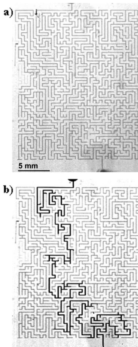
**Figure 1.** (a) A one-solution maze filled with a solution of bromophenol blue in ethanol. (b) The same maze after injecting a second solution of commercial food dye in a water/EG mixture into the inlet located at the top using a syringe pump. The purple stream found the way to the outlet at the bottom of the pictures.
