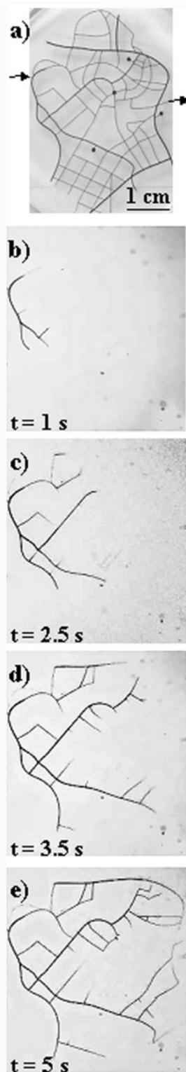
**Figure 7.** (a) Microfluidic network based on a map of Boston completely filled with an aqueous food dye in a water/EG mixture. Only some of the main streets of the city are included, with major arteries and interstate highways represented by larger channels than the smaller roads. (b–e) A solution of bromophenol blue in ethanol flowed into the network that was prefilled with a 1:4 mixture of water and glycerol. (e) Two routes emerged, with one being slightly faster.
