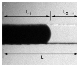
**Figure 6.** Black water-based ink displacing PFMD from a microchannel. The ink, which has a viscosity of  $\eta_1$ , occupies a length  $L_1$ ; the PFMD, which has a viscosity of  $\eta_2$ , occupies a length  $L_2$ . Note that  $L$  is the sum of  $L_1$  and  $L_2$ .
