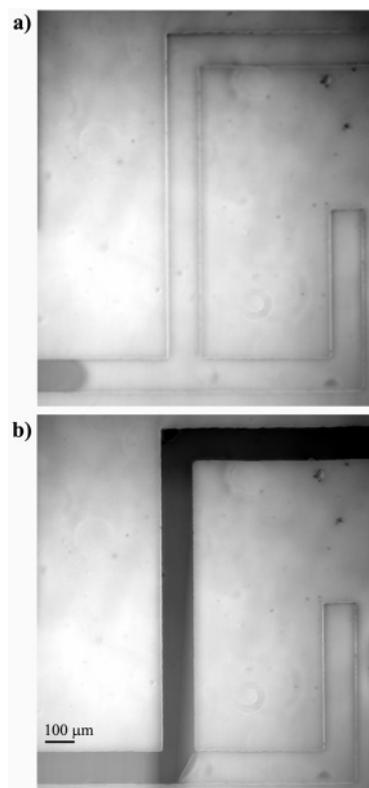
**Figure 2.** (a) Maze channels filled with PFMD (colorless). Ink displaced the PFMD from the left. The ink/PFMD interface was well defined and parabolic. Note that the path that continues to the right is a dead end, while the path that goes upward leads to the outlet. (b) The same channels after the ink had passed the intersection with the dead end. The PFMD did not flow into the dead-end channel.
