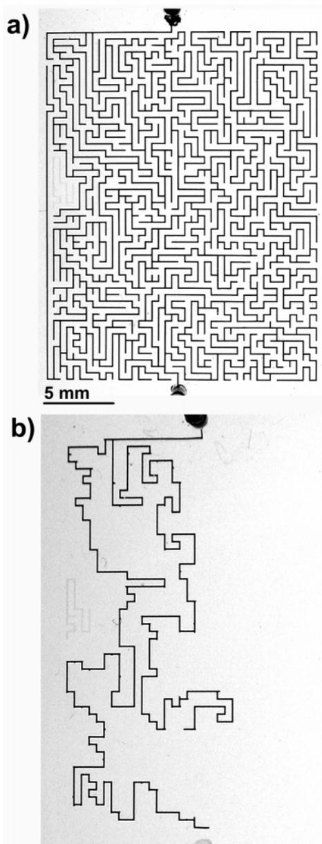
**Figure 8.** (a) A two-solution maze filled completely with an aqueous ink solution. (b) The same maze filled initially with PFMD, then injected subsequently with ink. The path that is filled completely with ink is 84.5 mm long, while the other path is 86.5 mm long. Due to the difference in viscosities of the two fluids used, the ink advanced only  $\sim 77$  mm into the longer channel.
